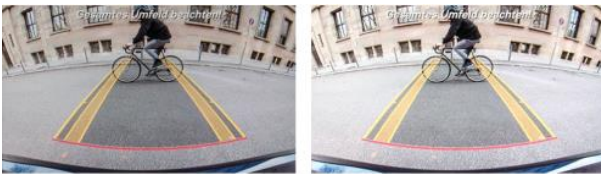
Figure 14. Even minor gamma distortions (right) are detected as “faulty reproduction”.
