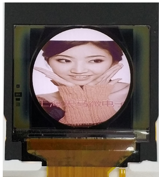
Figure 5. Image of the Demo with GIP and demux circuit based on IGZO TFT (transmissive mode)
