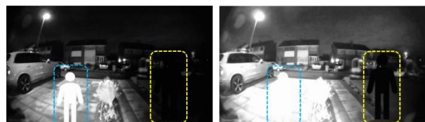
Figure 9. Visibility of bright and dark objects using short (left) and long (right) exposure time.
