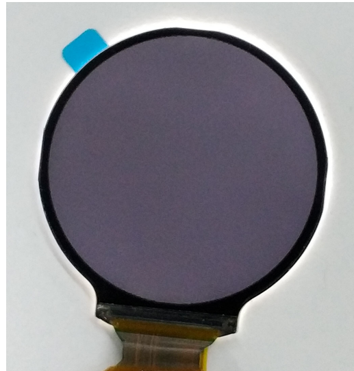
Figure 4. Image of the Demo with pin to pin design based on IGZO TFT
