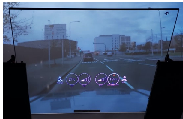
Figure 4: Holographic Windshield Cluster demonstrator built by Ceres Holographics and Texas Instruments
