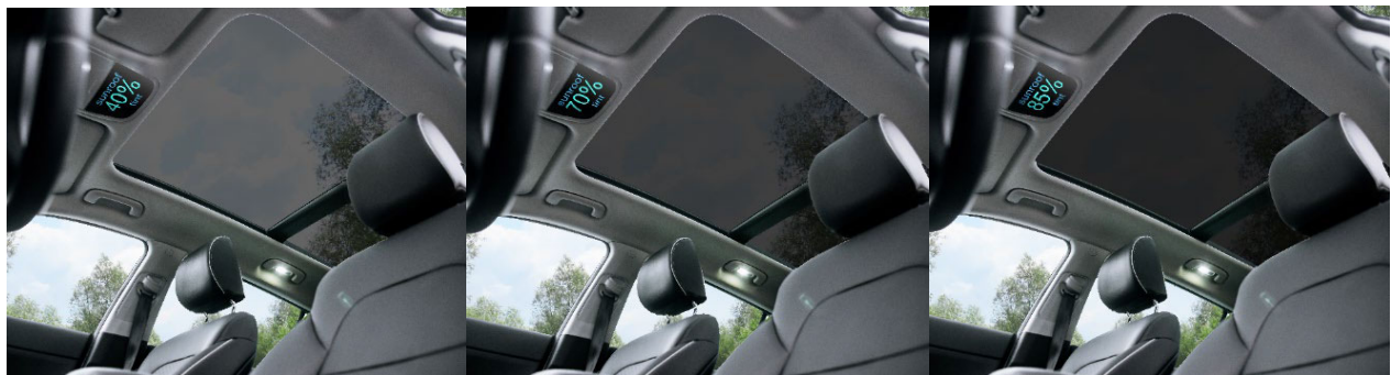
Figure 6: Concept of a smart window using Flexible liquid crystal cells. Image source: FlexEnable
