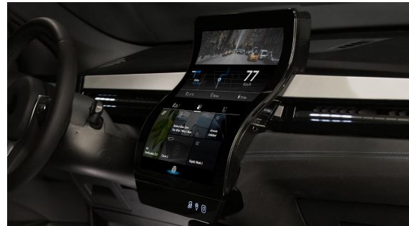
Figure 1. An S-shaped, touch-enabled centre unit consisting of twin 12.1" OLCDs. Image source: Novares
