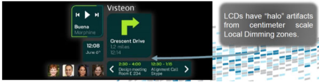
Figure 3. Local Dimming Zone Halo Depiction
