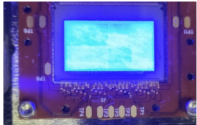
Figure 1. This close-up image of a microLED panel shows wide variation in luminance of different pixels across the display.
